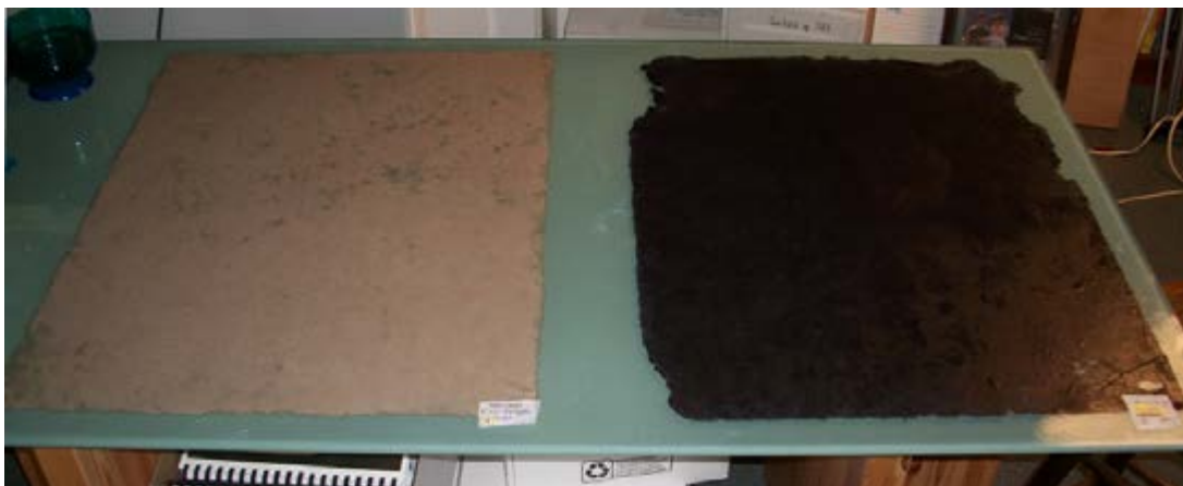
Figure 3. Two sheets of PC paper, drying on the glass. Each sheet is about 53 x 70 cm.
